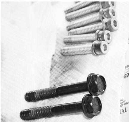
**5** After a thorough cleaning and a drop of 242 Loctite, the original bolts will be used to install the new Hayden M6 tensioner.
