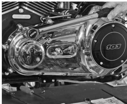
**16** After insuring that the long and short screws go where they belong and have each gotten a drop of Loctite 242, tighten them to 12-13 ft.-lbs.
