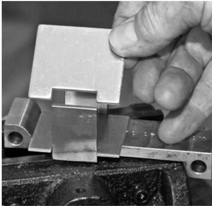
**12** If needed, one or both of the supplied shims can be inserted under the shoe to correct the installed spring height. Try the thin one first.
