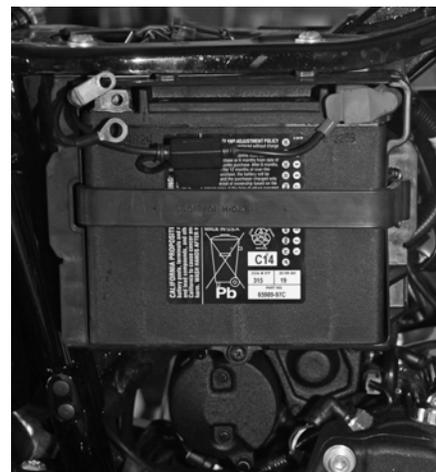
**2** But before removing the primary cover, disconnect the cables from the negative (-) side of the battery. Use a #2 Phillips screwdriver to remove the battery cover and a #3 Phillips to disconnect the cable.
