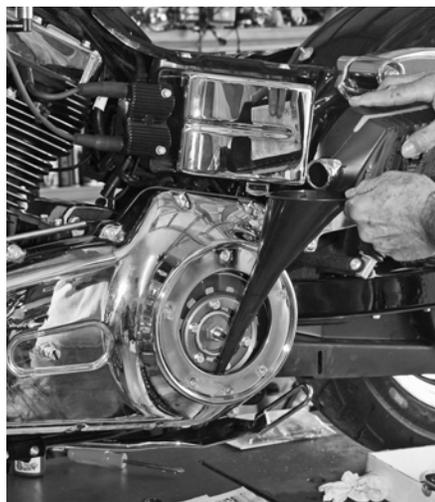
**17** Remove the derby cover screws with a T7 Torx and pour a quart of primary lube into the primary case. This is where you'll notice if you forgot to replace the drain plug.
