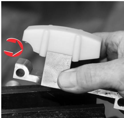
**7** The shoe and springs fit onto the guide plate as shown, with the curved relief in the shoe (arrow) facing the front of the bike.
