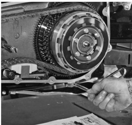
**14** The drain plug was wrapped with Teflon tape at the factory. I followed suit after installing a new O-ring. Tighten the plug to 14-21 ft.-lbs.
